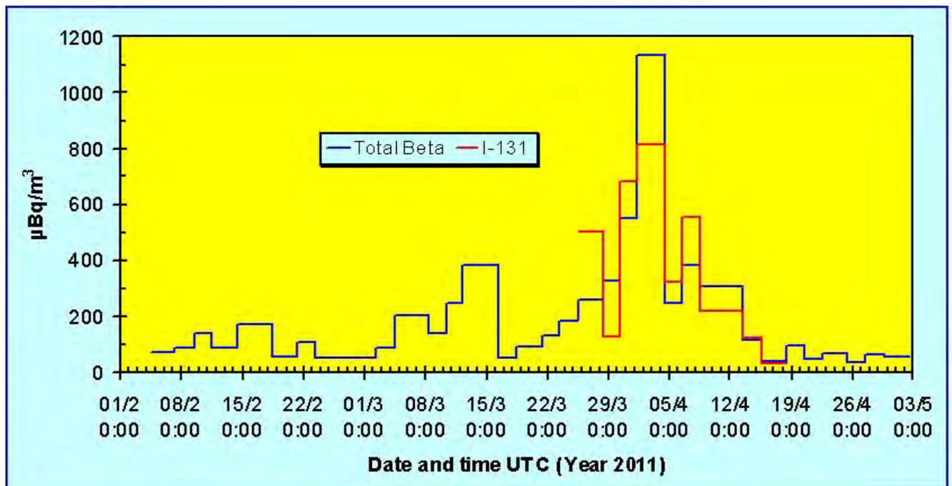
Figure 2. Total beta and  $^{131}\text{I}$  concentrations observed at Mt. Zeppelin in Longyearbyen, Svalbard (Figure adopted from Paatero et al., 2012).
